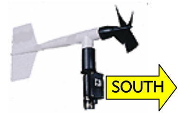
Propeller Style Black Junction Box Should Point in the South Direction
