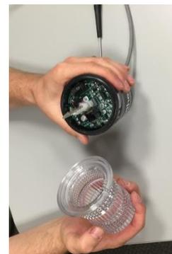
3. Remove the circuit board from the base by locating the two black clips and pinching them to release the board.
