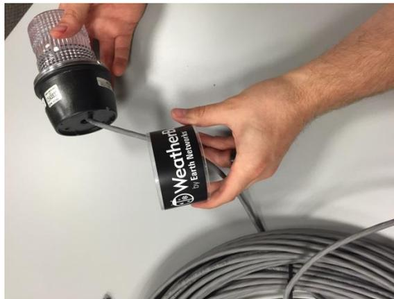
2. In order to secure the strobe to the ceiling or wall remove the clear cover of the strobe by unscrewing the small fastener screw and rotating the clear cover counterclockwise from the black base.
