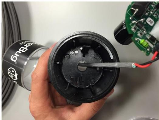
5. Once the base has been attached to the wall or ceiling, return the board to the base and clip back into place.
