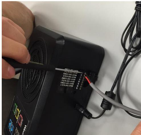
3. Connect the green connector on the opposite end of the short gray wire with the green connector on the 100 ft gray strobe cable.
